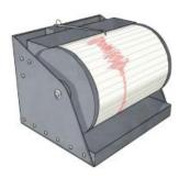
A seismograph (say: size-mo-graf) is a special piece of equipment that records earthquakes. Seismometers are securely fastened to the Earth, so when the ground starts to shake, the instrument's case moves too. What doesn't move is a weight that hangs on a string inside the case. When there is an earthquake, the case shakes with the ground but the weight does not, and it draws a line to show how much the ground shook.
